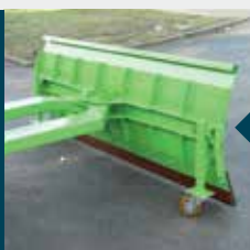
Tablier orientable 7 positions
